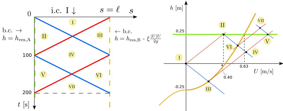
Figure 1: Question III.4:  $s, t$ -plane (left) and state diagram (right)
