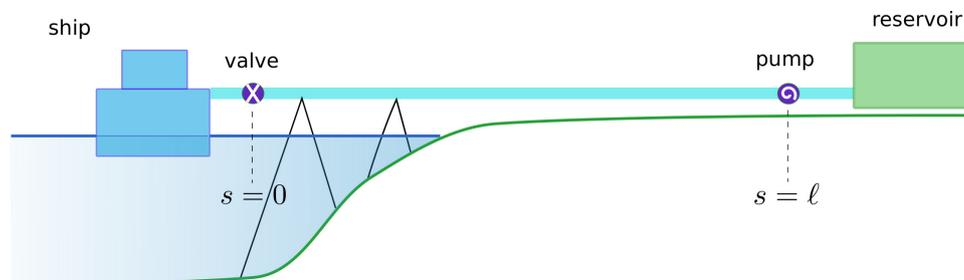
The pipe has a diameter  $D$  of 1.25 m, a wall-thickness  $\delta$  of 1.0 cm, and is made of steel with an elasticity modulus  $E$  of 200 GPa ( $= 200 \times 10^9$  Pa). Kerosine has a bulk modulus  $K$  of 1.3 GPa and a density  $\rho$  of 800 kg/m<sup>3</sup>.
