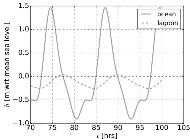
**III.2<sup>1.0</sup>** Explain how it follows from the above graph that the influence of inertia in the tidal inlet-lagoon system is negligible.
