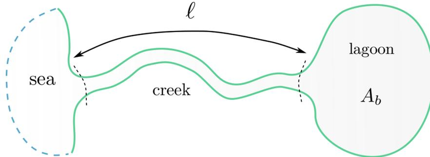
The response of the lagoon-creek system to the tidal forcing can be modelled using the so-called discrete system approach.
