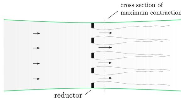
The expression for the corresponding resistance parameter reads  $\chi = \frac{1}{2}\mu^{-2}$ , in which  $\mu$  is the total contraction coefficient, i.e. the ratio of the conveying part of the cross section at maximum contraction and the total conveying cross section  $A_c$  of the bay inlet.
