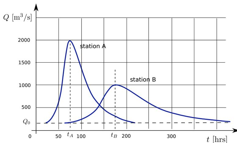
**IV.1<sup>1</sup>** Explain which feature(s) in the observed hydrographs is (are) typical of diffusive flood waves.
