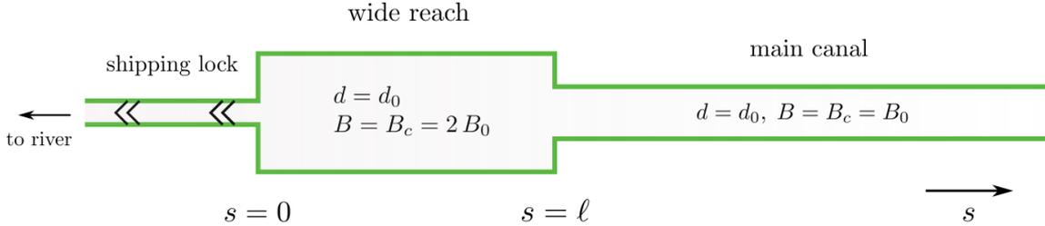
A levelling procedure starts at time  $t = 0$ , from which the water level in the lock is lowered with a constant rate of 60 cm/min. The lock chamber has a wet surface area of  $20 \times 100 \text{ m}^2$ . The canal has an undisturbed depth  $d_0$  of 2.5 m and the main canal width  $B_0$  (see figure) equals 40 m.
