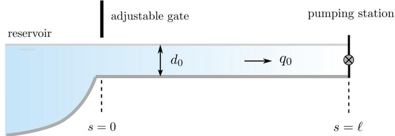
Manipulation of the gate and/or the pumping station in the above situation will cause transitory waves in the canal, superimposed on this initial flow state.
