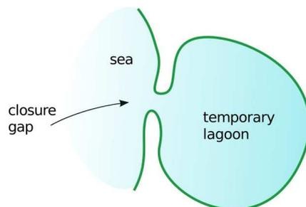
The configuration consisting of the lagoon and gap is modeled as a discrete system with storage and resistance.
