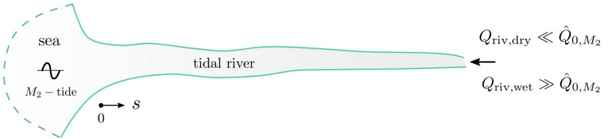
We will first consider the dry season with a low river discharge. In this situation the tidal wave in our river is a *progressive* wave. Generally, a progressive tidal wave occurs if the product of the damping parameter  $\mu$  of the tidal wave and the length  $\ell$  of the river is large.
