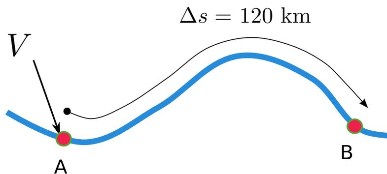
**IV.3<sup>1</sup>** Compute the travel time of the top of the high-water wave to a point B which is situated at a distance  $\Delta s = 120$  km downstream of A.
