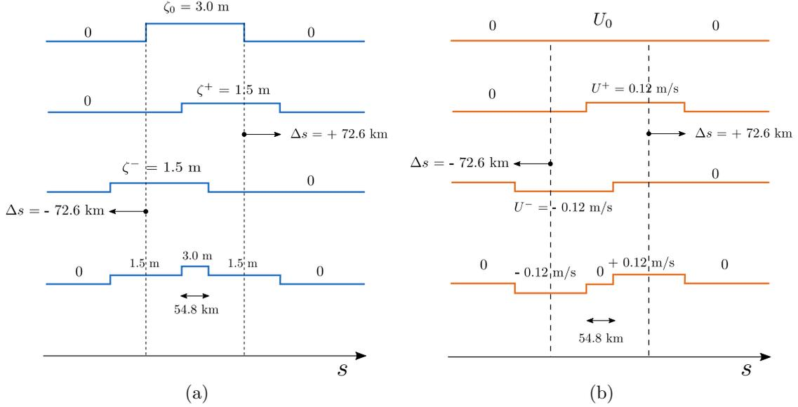
Figure 1: Question I.4: surface elevation (a) and flow velocity (b) at  $t = 600$  s
