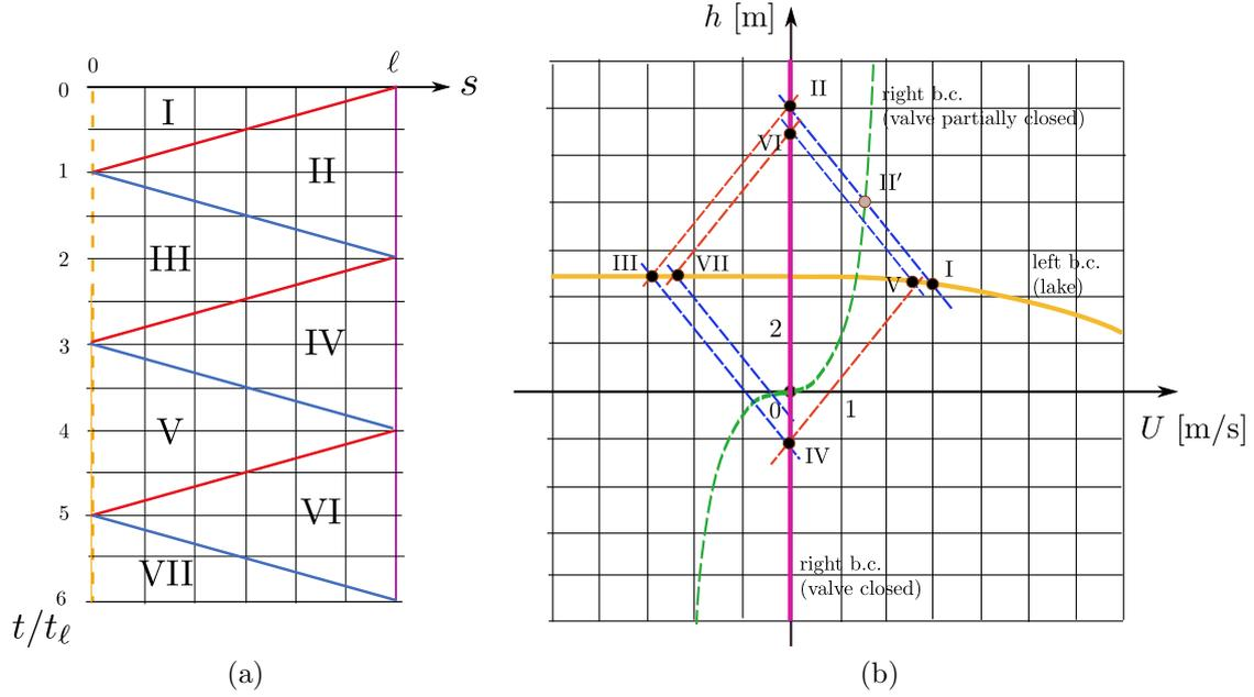
Figure 2: Question II.3:  $(s, t)$ -plane (a) and  $(U, h)$ -state diagram (b); characteristic relations are plotted schematically, not representing the correct slope
