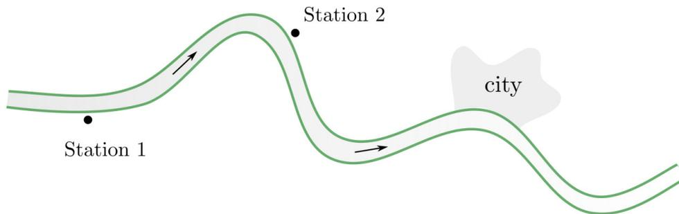
The predictions involve some calculations using a linearized model for high-water wave propagation in rivers. To this end, the river is schematized using a uniform width  $B = 3B_c = 600$  m, a uniform bed slope  $i_b = 2 \cdot 10^{-4}$ , and a uniform resistance coefficient  $c_f = 4 \cdot 10^{-3}$ . The peak of the wave travels in 12 hrs from Station 1 to Station 2, which is a streamwise distance of 35 km.
