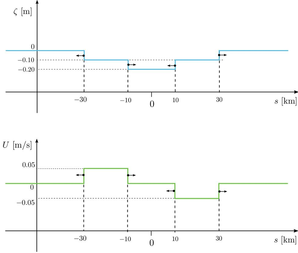
Solution of Question I.3; arrows indicate propagation direction of the respective wave fronts
