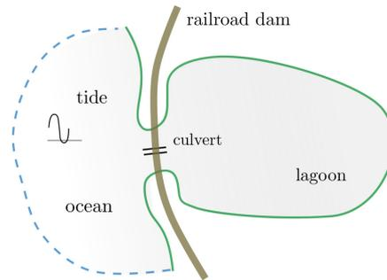
The response of the lagoon and its inlet to the ocean tide is similar to the response of a mass-spring-damper system to a periodic forcing.
