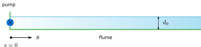
At time  $t = 0$  the pump is switched on with the specific discharge  $q$  gradually increasing in time to  $0.20 \text{ m}^2/\text{s}$ , which results in a singular translatory wave in the flume.
