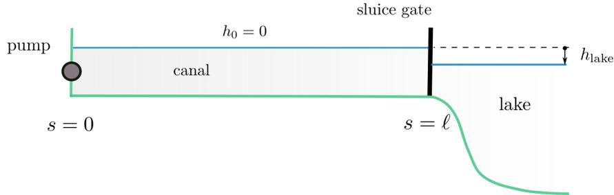
The canal has a cross section  $A_c$  of  $25 \text{ m}^2$  and a storage width  $B$  of  $10 \text{ m}$ . At time  $t = 0$  the sluice gate is opened partially while the pumps are still off. As a result, a negative transitory wave is issued into the canal with a height of  $-0.25 \text{ m}$ .
