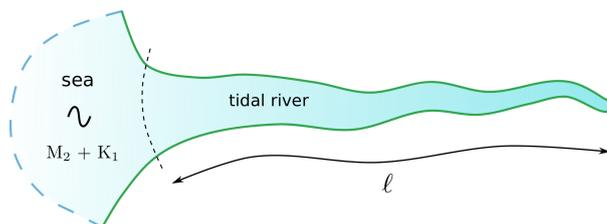
**II.1<sup>1</sup>** Describe, in general terms, the influence of the frequency on the propagation of *progressive* harmonic waves in a uniform channel with constant linear friction factor.
