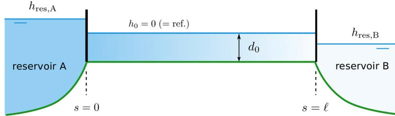
At time  $t = 0$ , the gate at reservoir A is opened fully and abruptly. This results in a positive translatory wave in the canal with a specific discharge  $q$  of  $1.5 \text{ m}^2/\text{s}$ . In- and outflow losses, and other effects related to the local velocity head can be neglected for this gate.
