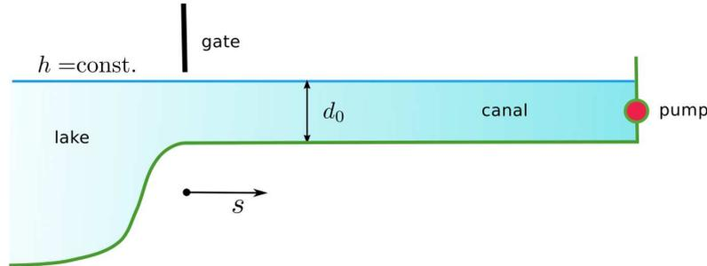
In this question the wave motion in the canal resulting from manipulations with the pump and/or gate will be studied using the elementary wave equation.
