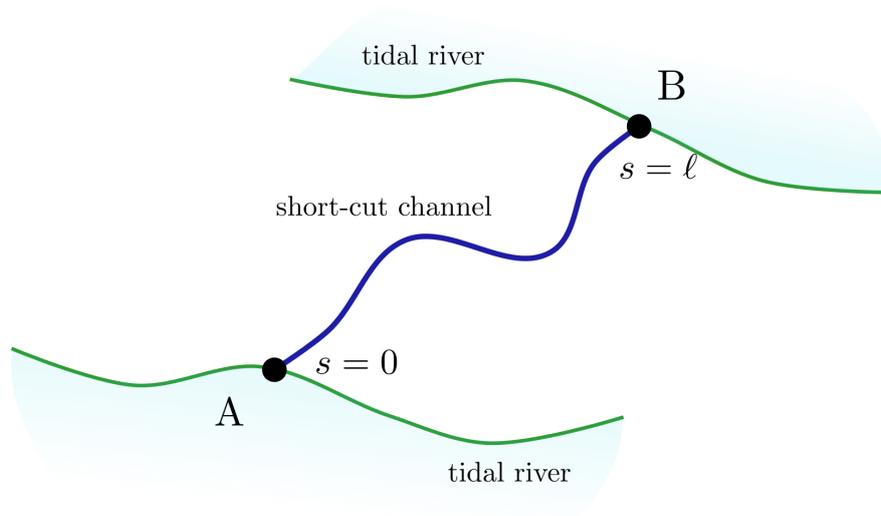
The short-cut channel has a length  $\ell$  of 55 km. Its cross-section is approximately uniform with a conveying cross-section  $A_c$  of 800 m<sup>2</sup> and a storage width  $B =$  of 300 m.
