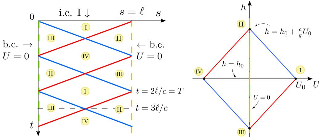
**II.4** The state in the pipe repeats after  $t = 2t_\ell$ , so the period of the periodic motion is given by  $T = 2\ell/c = 2.0$  s. The amplitude of the piezometric level is given by  $\hat{h} = h_{II} - h_0 = h_{II} - h_I$ . Using the characteristic relation  $dh/dU = -c/g$  from state point I to point II (positive characteristic), and using  $dU = U_{II} - U_I = -U_0$ , it follows that  $dh = h_{II} - h_I = +U_0 c/g$  giving a piezometric level amplitude of  $U_0 c/g = 120.8$  m.
