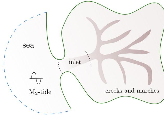
The most important element of the design is the surface level amplitude inside the wetland which, apart from the tide at sea, depends on the wet surface area of the creeks and marshes in relation to the properties of the inlet. For this wetland, it can be assumed that all its components are small relative to the tidal wave length, and that the role of inertia in the resulting tidal system is negligible.
