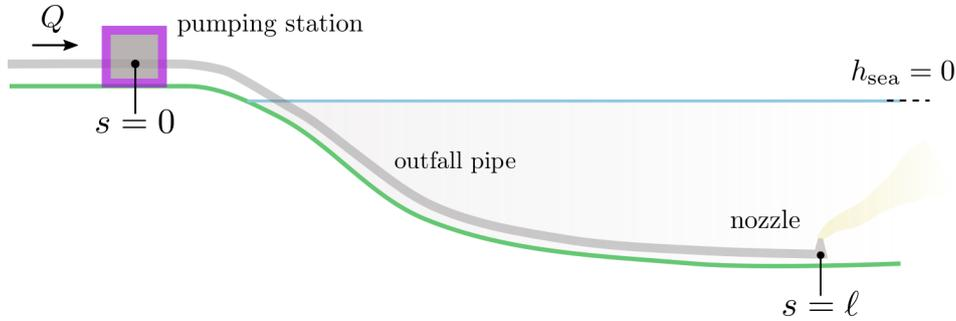
In the past, several such outfall pipes have collapsed due to the formation of vapour bubbles in the pipe caused by extremely low fluid pressures.
