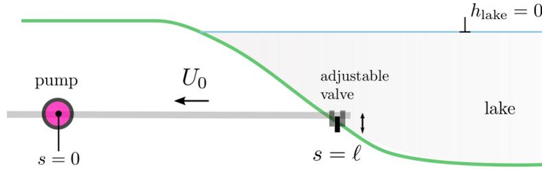
The pipe is made of GRP ( $E = 17$  GPa) with a length  $\ell$  of 1,500 m, an inner diameter of 1.2 m, and a pipe-wall thickness of 0.02 m. The bulk modulus of water ( $K$ ) equals 2.2 GPa.
