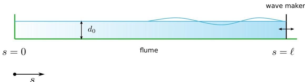
The wave generator is switched on. The horizontal, sinusoidal motion of the paddle generates periodic harmonic waves in the flume with a period  $T$  of 5 s. The undisturbed depth  $d_0$  in the flume equals 30 cm.
