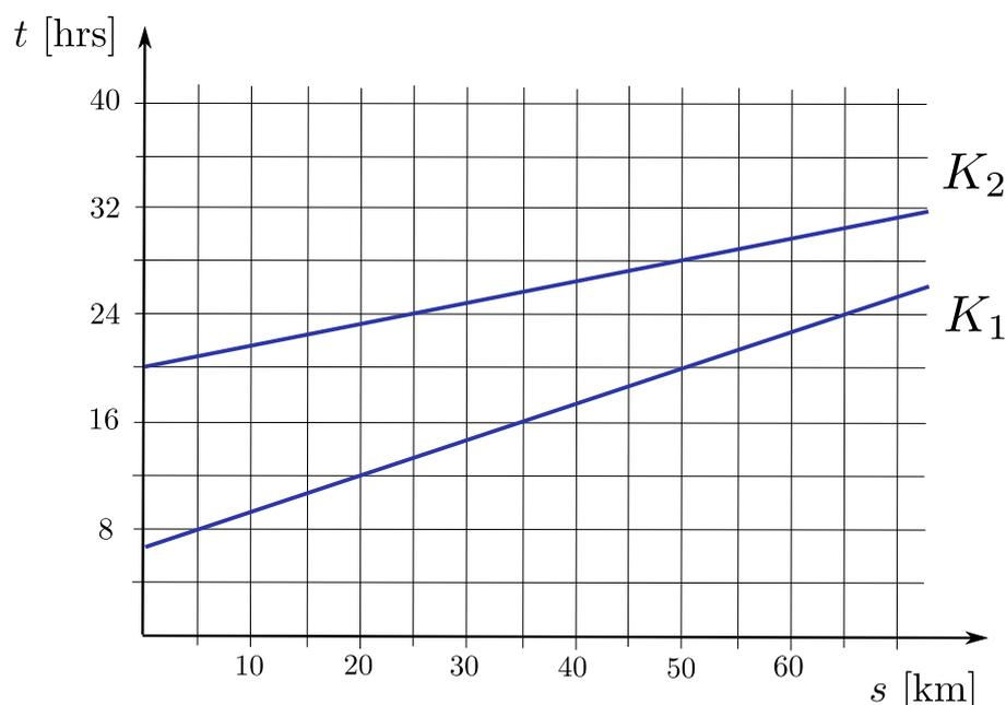
**IV.2<sup>1</sup>** Explain why the characteristics of a kinematic flood wave in a uniform channel are always straight lines.
