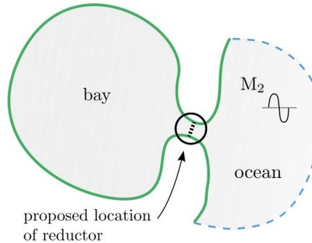
The tidal basin has an undisturbed depth  $d_0$  of 6 m, a surface area  $A_b$  of  $80 \text{ km}^2$ , and horizontal dimensions of approximately  $9 \text{ km} \times 9 \text{ km}$ .
