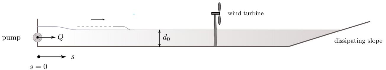
Starting from rest, the compression wave is generated by gradually increasing the discharge at the entrance of the flume. The compression wave steepens until it breaks.
