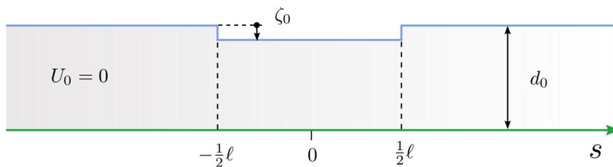
The undisturbed depth  $d_0$  amounts to 40 m, the initial surface displacement  $\zeta_0$  equals  $-0.20$  m, and the wavelength  $\ell$  equals 40 km.
