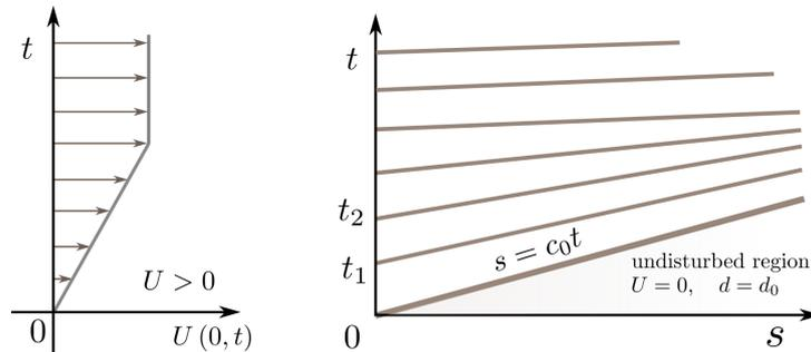
Figure 3: Compression wave: velocity variation at inflow boundary (left) and  $(s, t)$  diagram showing the positive characteristics (right)
