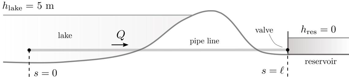
The concrete pipe has a uniform cross section and is infinitely rigid. Experience with similar intake pipes has shown that too abrupt changes of the discharge can cause structural failure of the pipe.
