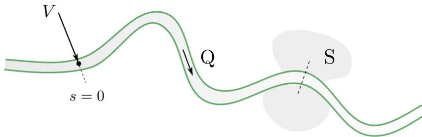
The top of the flood waves passes the settlement  $S$  at time  $t_S = 8 \text{ hrs}$  after the occurrence of rainfall.
