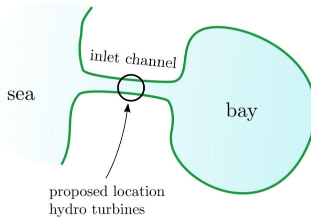
The bay-inlet system can be modeled as a so-called *discrete system*.
